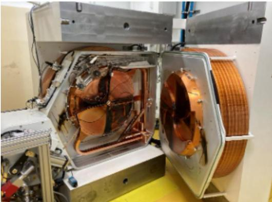
*A cyclotron is a particle accelerator machine that uses electromagnetic fields and RF signal to propel charged particles to very high speeds and energies, used to produce radioisotopes, such as  $^{18}\text{F}$ , which are essential / core components of radiopharmaceuticals.*
